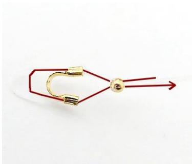
1) Insert 1 brass crimp bead, 1 wire guardian on the thicker wire the 0.20 for about 1,60 m
